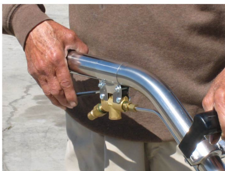
image 3A, 3B Press the lever to open the valve
